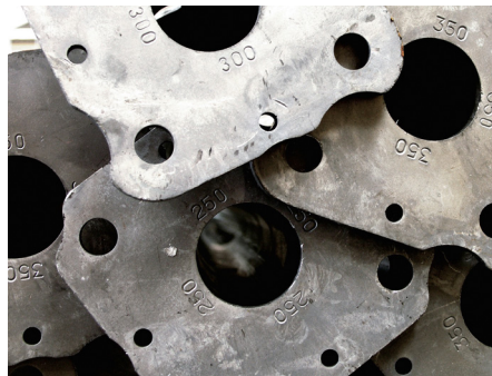
The length stamping on the PEP Ergo props is clearly readable.
